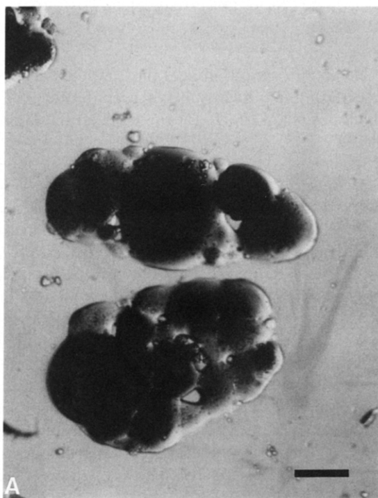
Fig. 4. Degradation of microspheres at the onset of collapse. The micrographs show the microspheres just before (A) and after (B) collapse. Bar, 100 \mu m.
